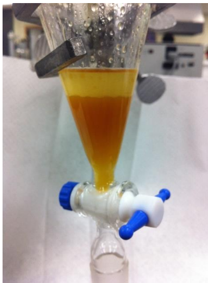
Figure 2. Crude product was extracted with Ethyl acetate
